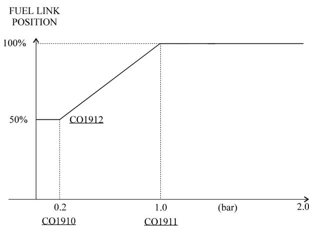
The torque limiter monitors the engine speed and position of the fuel rack to prevent excess torque being developed by the engine, which would thermally overload the engine and hence increase combustion chamber stresses.
