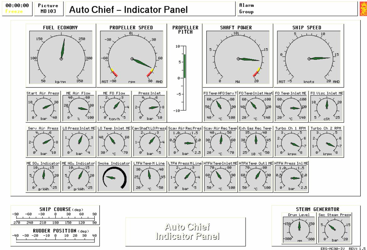
The indicator panel provides the operator with an overview of the main parameters that influence the main engine. Each of the gauges readings can be located on their individual operating or control screens.
