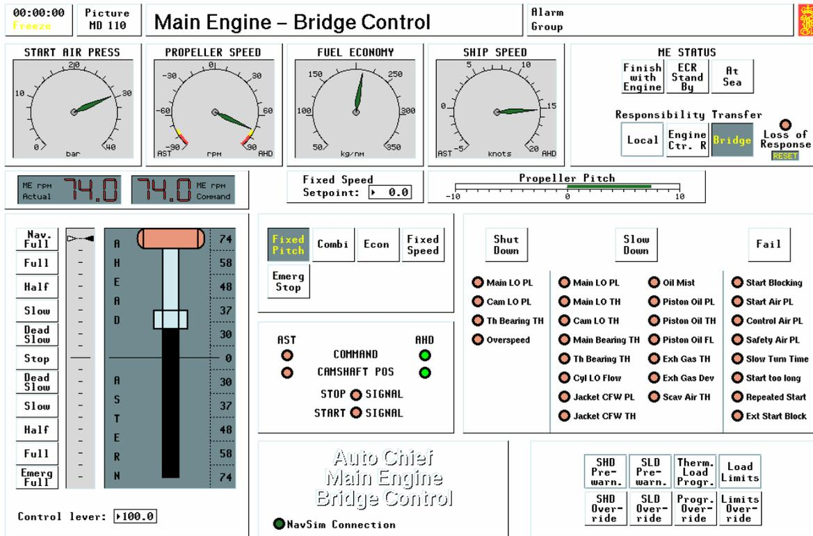
The control system fitted to the bridge is a mimic of that fitted within the Engine Control Room. Both panels have the same functionality, although some minor controls are different. Note that the Bridge has a starting air pressure gauge, which is mandatory for all engine manoeuvring positions.
