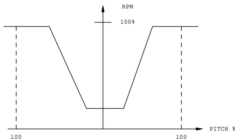
At zero pitch the engine speed is reduced to improve manoeuvrability, and as the fuel control lever is increased, then the pitch and engine speed increases until the engine is
