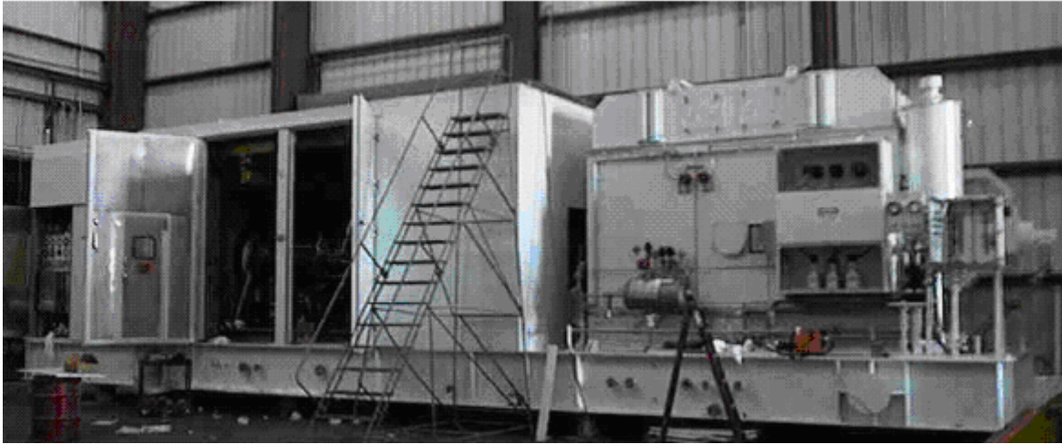
Figure 10 Gas turbine and generator assembly
