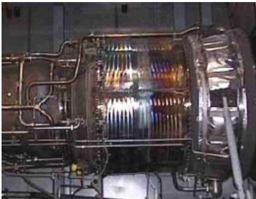
Figure 14 Power turbine element
