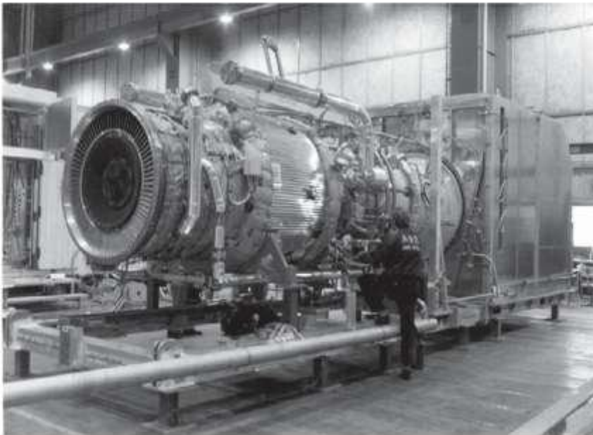
Figure 31.11 One of two 17 000 kW Alstom Power GT35 gas turbines supplied to drive the waterjets of a Stena HSS 900-class fast ferry
