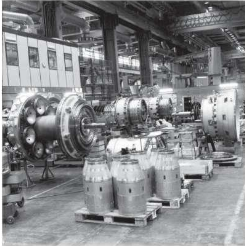
Figure 31.13 Seven large can-type combustion chambers (foreground) contribute to the lower grade fuel burning capability of Alstom Power's GT35 turbine.
