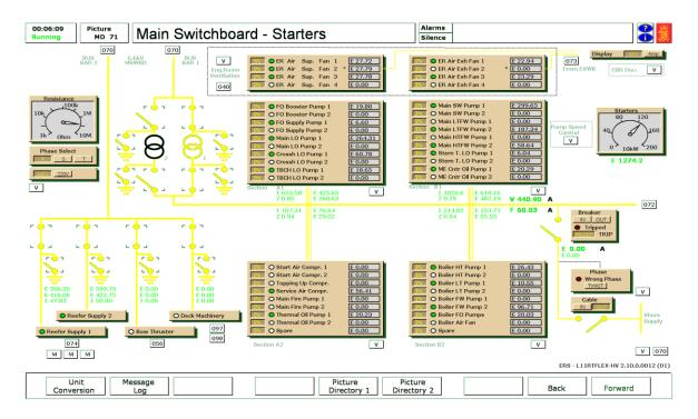
Bus bar 1 powers all the electrical main consumers and the emergency bus bar. Bus bar 2 powers the bow thruster and deck machinery.
