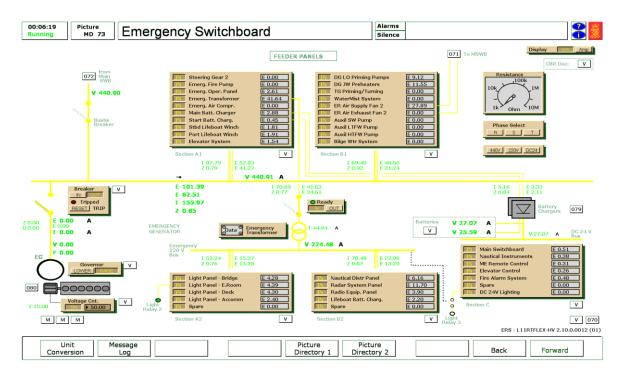
The emergency switchboard supplies circuits necessary for the safety of the vessel. These include communications, navigation lights, fire alarm, fire and flood control etc.
